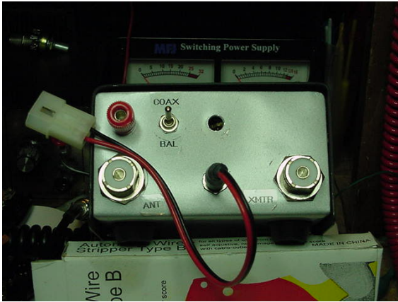
Tuner backside with power for bargraph
